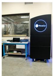
When operated in HIL mode, the RTDS executes power system models in real time, directly supporting controller design and testing. In PHIL mode the RTDS interacts with real hardware such as energy storage systems, loads, and distributed energy sources by driving them through power amplifiers. The hardware's dynamic response is then fed back into the simulation loop, creating a fully integrated cyber-physical test environment for power systems.
