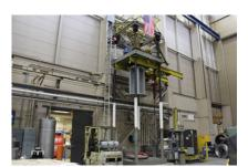
**Assembly Press** - The primary hydraulic composite assembly press in the high bay is 40 ft tall and is capable of generating forces in excess of 500 tons with room for 20 - 25' parts and a 60 in. stroke, one smaller 200-ton H-press with 13 in. stroke, one smaller 200 -ton hydraulic four-column assembly press.
