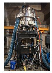
The dynamometer is bi-directional and is capable of both vertical and horizontal orientation; this is critical for testing of vertical axis motor/generators for advanced energy storage flywheels. The electro-pneumatic inlet and outlet control valves control the flow of water to the dynamometer based on commands from the Kahn Series 545 digital dynamometer controller. The hydraulic dynamometer provides a controlled load for a prime mover such as a gas turbine or electric motor..
