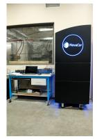
Digital Real-Time Simulator - The lab features both an RTDS (Real-Time Digital Simulator) Novacor 2.0 and an OPAL-RT real-time simulator, enabling high-fidelity, real-time simulation of complex power systems. These platforms facilitate closed-loop interaction with physical controllers and relays, supporting the development, validation, and de-risking of advanced control systems under realistic operating conditions.
