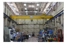
**Overhead Cranes** - Two 25 ton overhead cranes for main high bay area, additional 25-ton overhead crane for machine shop, smaller 3-ton crane in auxiliary machine shop.
