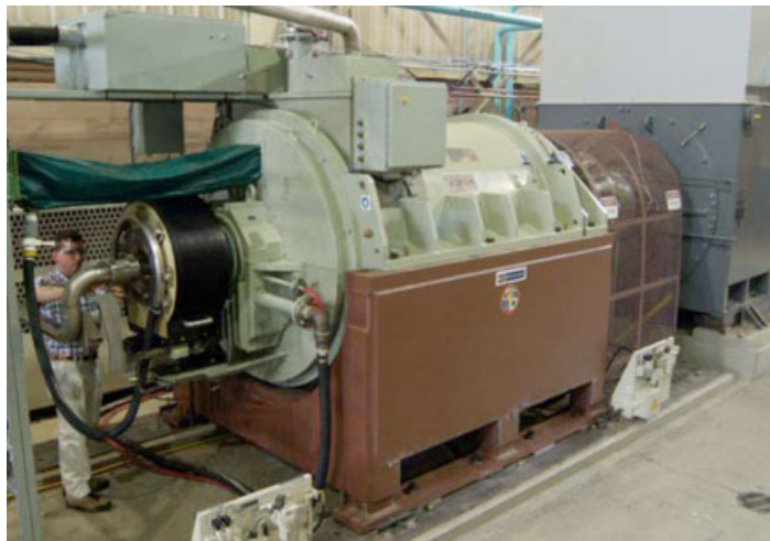
Figure 3: American Superconductor Co.'s 5 MW HTS synchronous motor under test.
